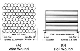
This lost area is *made up of the space between the* wires and the insulation with which each wire is coated. As the voltage stress of the winding is increased, it is often necessary to add inter-layer insulation creating more lost space, thus decreasing the available conductor area.
